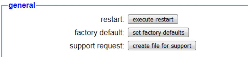
In the “general” area you can restart your device as well as setting the device back to it's factory defaults. To execute the action you have to click on the corresponding button.
