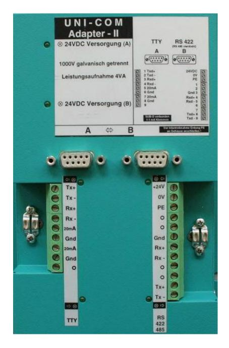
green LED: channel A is supplied with 24V DC green LED: channel B is supplied with 24V DC
