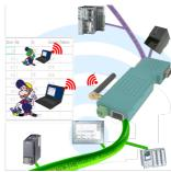
Wired or wireless communication (WIFI) via the same adapter with the respective control Devices from the BRIDGE-family always connect a wired-network with a wireless-network (WIFI) and a specific PLC-interface. This gives you access to the directly connected controller via WIFI (with S7 to the entired bus) as well as to the wired Ethernet. Of course also from wired Ethernet to WIFI and control/bus.
