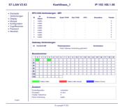
View information from the connected bus-system in plain text without using the Simatic-Manager or TIA-Portal. With the connection-menu you get the list of reachable nodes, marked in color whether it is an "active bus-participant", is a "candidate for inclusion in the bus" or a "passive bus-participant".
