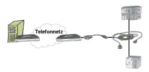
You have to reach urgend your PLC via remote maintenance and have no TS-adaptor in your company? No problem, configure with the MPI-Kabelmanager your S7-interface-cable MPI-II-Kabel the mode "TS" for "remote maintenance", connect this cable with the TS-Adapter (article number 9350-TS) with a standard modem and send it all to your client. Now you will be able to start the connection with your TS-sofware and solve the problem. And this all without buying a original TS-adapter.
