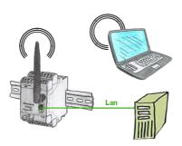
Access parallel via LAN and Wifi to the EtherSens-device. Therefor create via the web-server for each way an ip-address, regardless whether its the same subnet or not.
