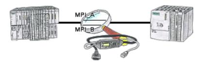
The S7-LAN can also be used for controlling/checking the MPI/Profibus. It will be plugged on the Bus so that you can take a look at the status of the busses via software on PC, for example the numbers of parity errors.
