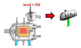
Do you monitor processes and upon reaching a predetermined upper/lower limit, you need a message? Then activate in the device the limit-value-monitoring and you get this message. Furthermore, the device also sends its state and you are always up to date.
