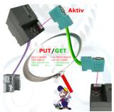
Direct data-exchange between S7-PLCs with S7-LAN.
